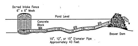
into the pipe so they won't block it. This creates a permanent leak in the dam. The height of the pipe in the dam controls the water level. The pipe inlet usually needs 3 feet of water depth to fool the beavers.
