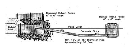
As seen in the diagram, the domed intake fence is sunk in the pond and is built large enough (usually 5-5.5' diameter) so that the beavers cannot feel or hear the water flow into the pipe. The Fence and Pipe device
