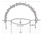
The Diversion Dam is inexpensive and relatively easy to build. It has an 80% success rate. Basically you create an easier place for beavers to dam located 10 to 15 feet upstream of the culvert. As shown in the diagram, it can be constructed in a semicircle and can be made from of any kind of material (fencing, rocks, etc.) that encourages the beavers to dam there rather than the culvert. It works best if it holds back some water like a small beaver dam. It can be built to allow wildlife passage.
