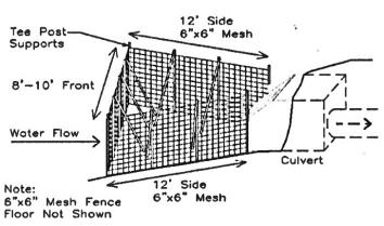
culvert the opening the water flows into widens so the damming stimuli of the sound and feel of moving water decreases the more they dam. This design is ideal for shallow water or high flow streams, but needs quarterly maintenance to remove floated debris.
