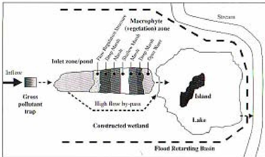
*This is a wetland constructed for stormwater detention and pollution control.
