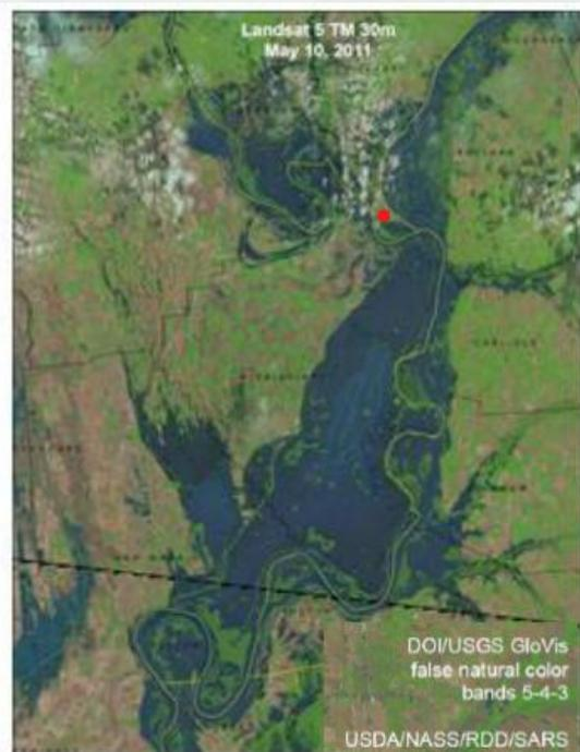
The purpose of the floodway is to lower flood stages upstream and adjacent to the floodway during major flood events. The Floodway is some 35 miles in length and varies from 4 to 12 miles in width. It comprises about 205 square miles of alluvial valley land.
