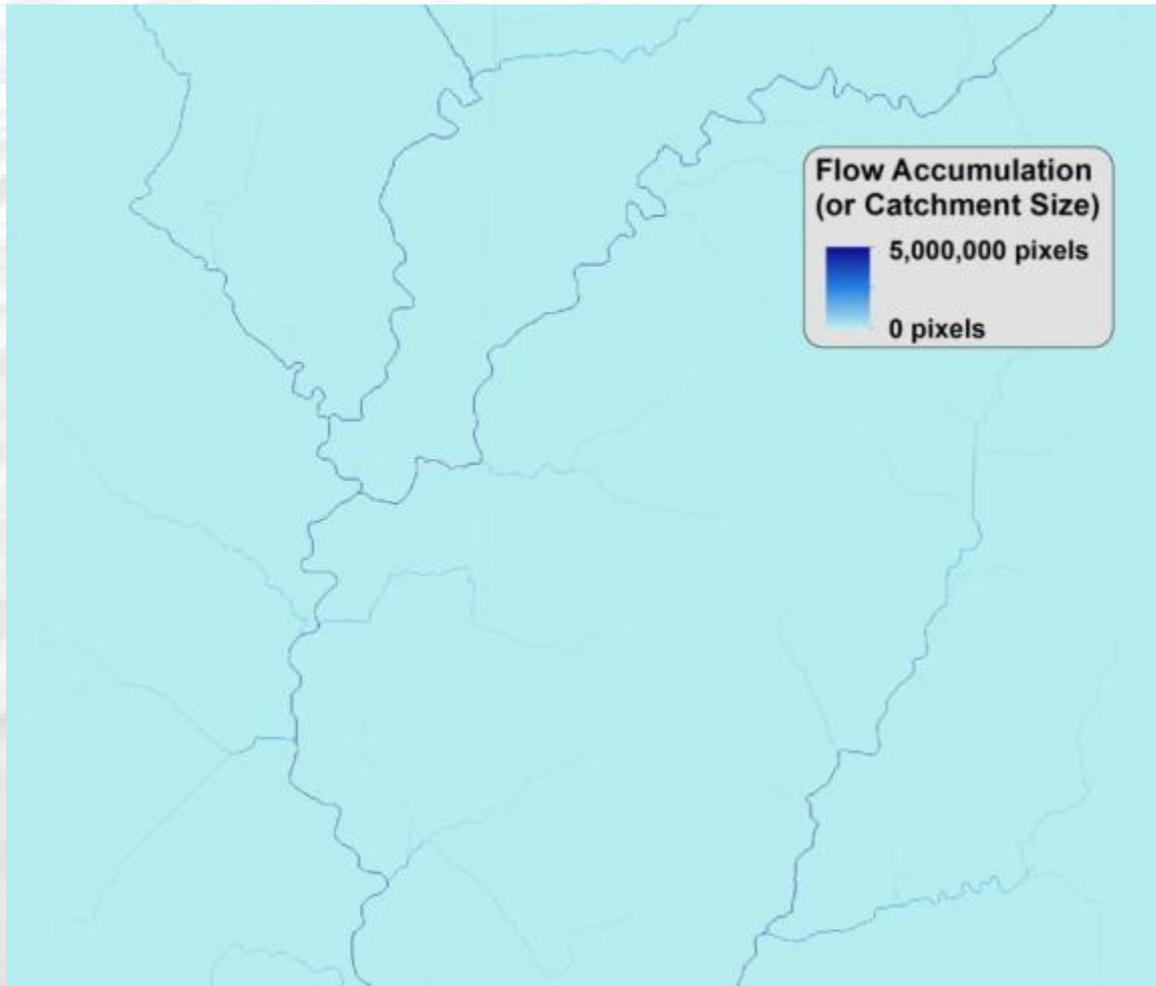
The flow direction map is used to compute flow accumulation.
