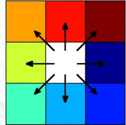
Each pixel is colored based on its flow direction.
