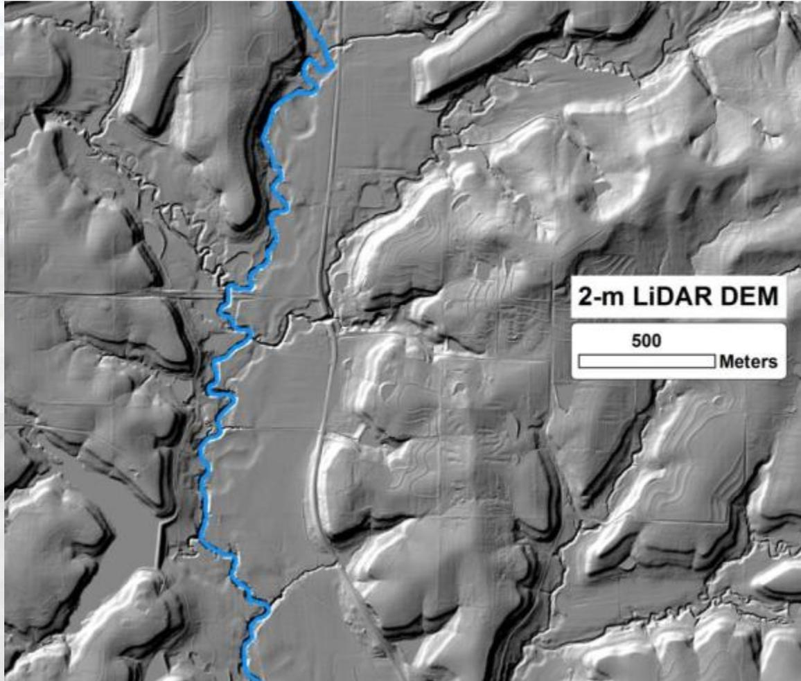
Using pixels with a flow accumulation value  $>10^6$  pixels, the **Mud Creek** streamline is identified (shown in blue).
