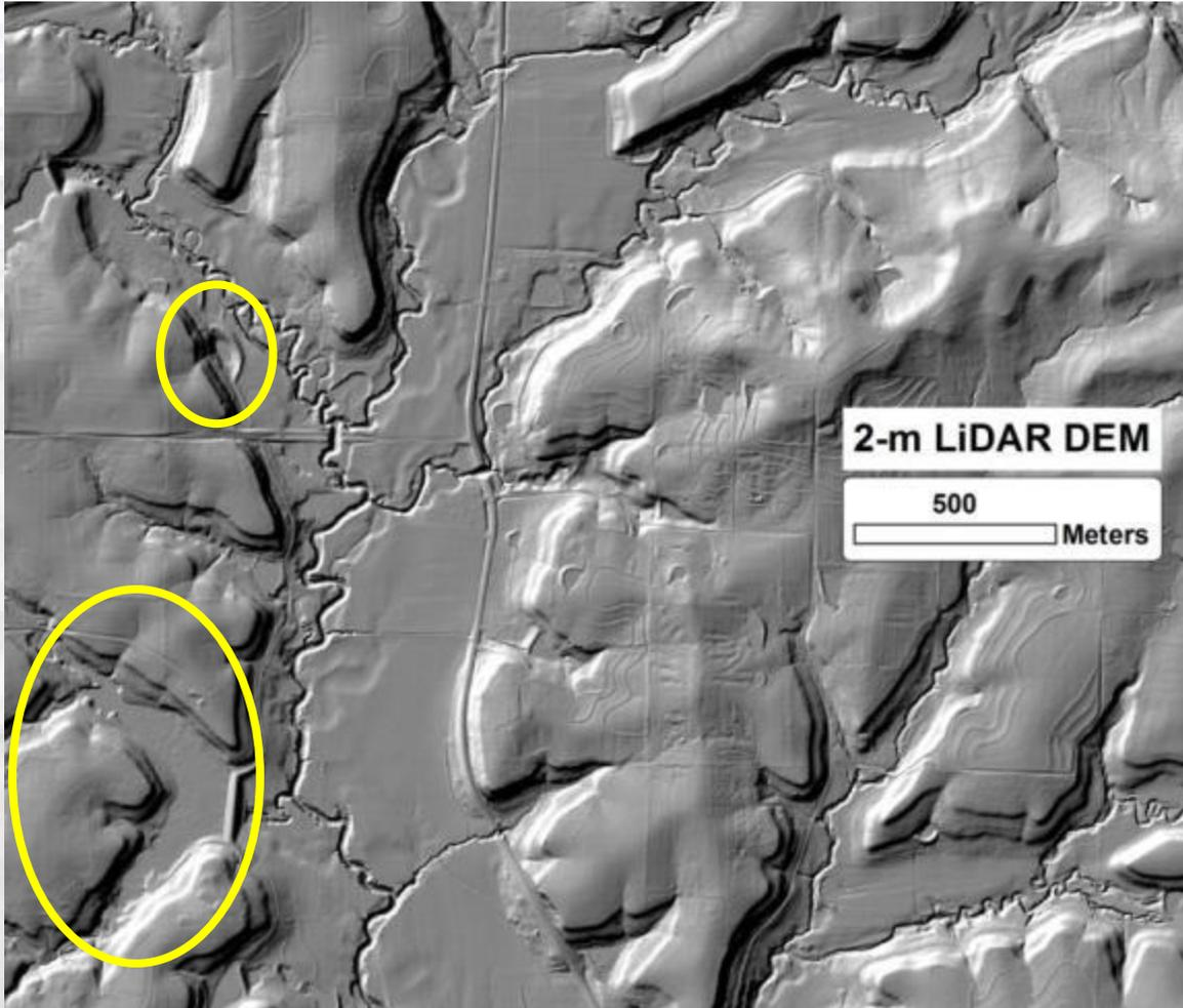
This DEM was created using LiDAR data.
