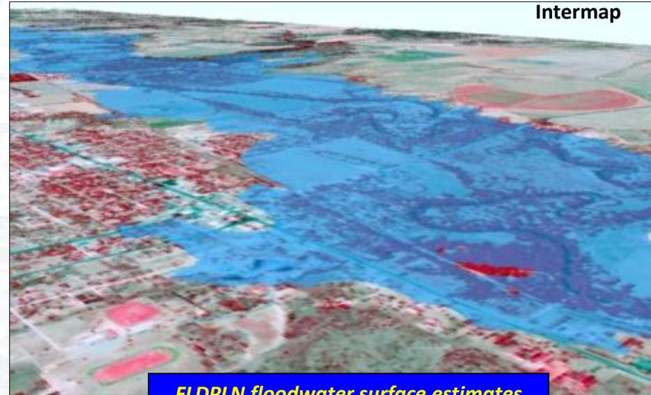
*FLDPLN floodwater surface estimates using different elevation datasets*
