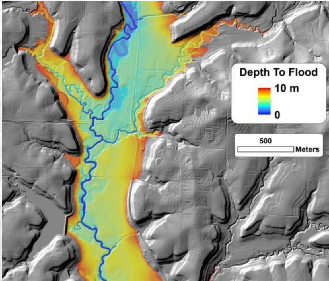
The 10-m floodplain was computed *for Mud Creek* using the FLDPLN model.
